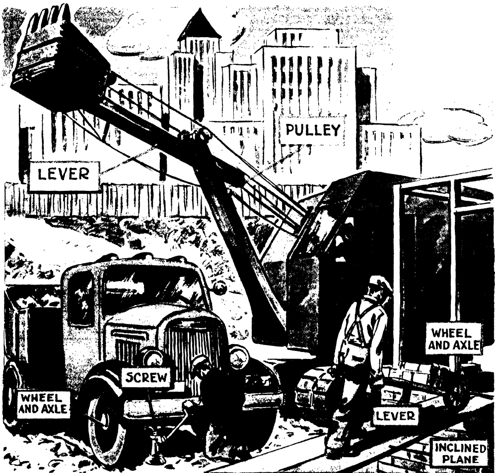
10. This drawing will give you some idea of the way in which machines are used on an ordinary construction job.
