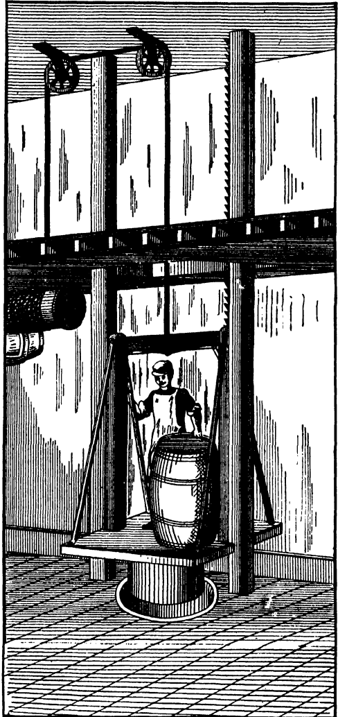
Culver Service An old-fashioned hydraulic (water-power) elevator, which worked with a plunger device in a cylinder.
