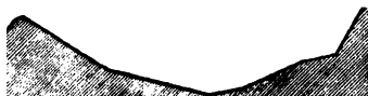
FIG. 57.—Section of Loch Goil, a typical rock basin, the slopes exaggerated 10 times. The upper line shows by its varying thickness the true slope of the bed of the basin.
