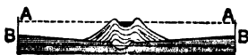
FIG. 54.—Embankment of a river. B B, original slope of valley. The light shading shows successive layers of deposit; A A, level of river.
