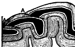
FIG. 48.—Production of thrust-planes A. The strata represented are layers of clay and sand separated by cloth; they were laid down horizontally, and ridged into the position shown by a thrust acting in the direction of the arrow. (From a series of experiments by Mr. H. M. Cadell.)
