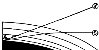
FIG. 21.—Atmospheric Refraction. A, observer; S, true position; S', apparent position of Sun. The density of the atmosphere is indicated by the closeness of the lines.
