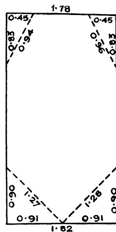
FIG. 7. SURVEY OF STRAIGHT-SIDED PLOT BY CORNER TRIANGLES
