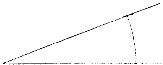
FIG. 22. SETTING OUT ANGLE WITH SCALE OF CHORDS
