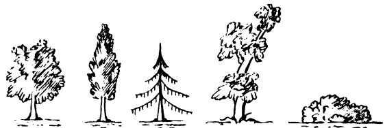
FIG. 28. ENLARGED SKETCHES OF TREES AND BUSHES ON SURVEY PLANS
