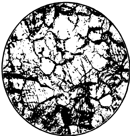
FIG. 3. PHOTOMICROGRAPH OF CARRARA MARBLE Showing crystalline calcium carbonate
