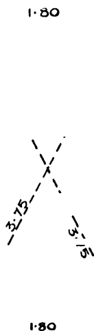
FIG. 6. SURVEY OF STRAIGHT-SIDED PLOT BY DIAGONALS
