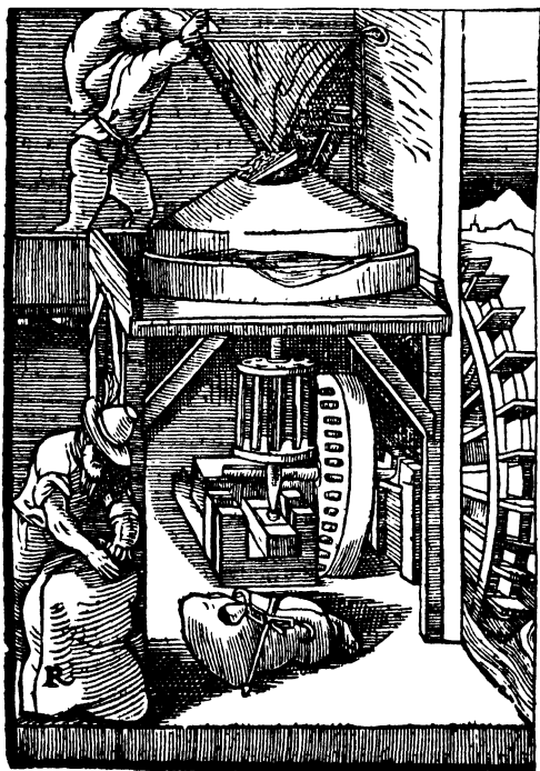
Fig. 10. Reconstruction of Vitruvius' water-mill.
