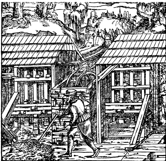
Fig. 20. A sixteenth-century water-driven stamp-mill for crushing ore.
